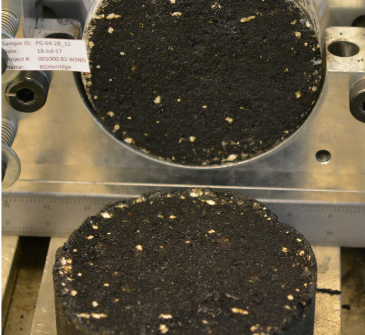
Photo 4: Specimen without waterproofing membrane, after shear testing. The light-gray spots on the shear interface are interlocked aggregate that abraded or fractured during testing.
