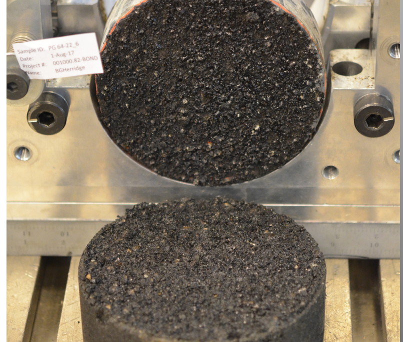
Photo 5: Specimen with waterproofing membrane, after shear testing.
